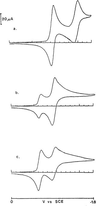
Figure 1. Cyclic voltammograms for 2 (a) in the absence of  $Li^+$ , (b) in the presence of 0.5 equiv of  $Li^+$ , and (c) in the presence of 1.0 equiv of  $Li^+$ .
