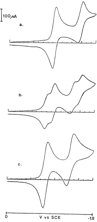
Figure 2. Cyclic voltammograms for 4 (a) in the absence of  $Na^+$ , (b) in the presence of 0.5 equiv of  $Na^+$ , and (c) in the presence of 1.0 equiv of  $Na^+$ .
