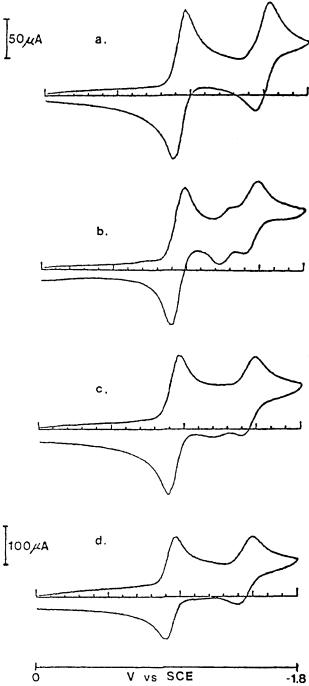
Figure 5. Cyclic voltammograms for 1 (a) alone and in the presence of 0.5 equiv of  $K^+$  using scanning rates of (b) 100 mVs<sup>-1</sup>, (c) 500 mVs<sup>-1</sup>, and 1000 mVs<sup>-1</sup>.
