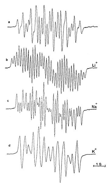
Figure 6. ESR spectra of  $4 (10^{-4} \text{ M in THF})$  (a) in the absence of cations and in the presence of 1 equiv each of (b) Li<sup>+</sup>, (c) Na<sup>+</sup>, and (d) K<sup>+</sup>.
